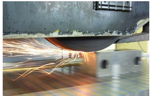
Surface grinding Magnetic table, 600 x 250 mm
