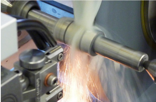
Cylindrical circular grinding Ø 0.5–100.0 mm, length 420.0 mm, Dimensional control
