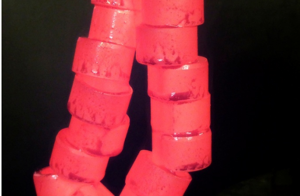
Hardening Salt bath hardening: through and surface hardening/tempering Max. dimension: length 40 cm width 20 cm
