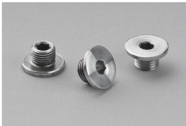
Centering screw D: M5x0.5 x 4.5 / M: 1.7225
